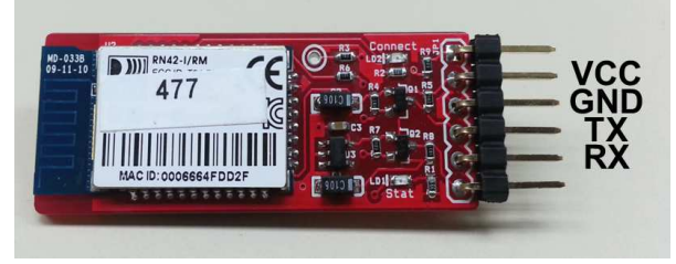
Figure 3. Pin Composition of the Bluetooth Serial Communication Module (RN-42 Silver)
