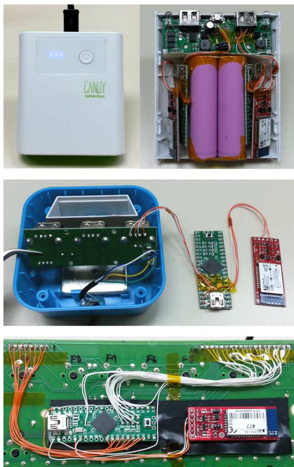
Figure 5. USB Device attached with IRON-HID - Portable Charger (top), Card Reader (center), Keyboard (bottom)
