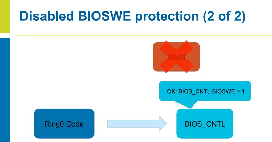
An SMI is generated on the write as before, but this time SMM just immediately returns instead of resetting the BIOSWE bit to 0.
