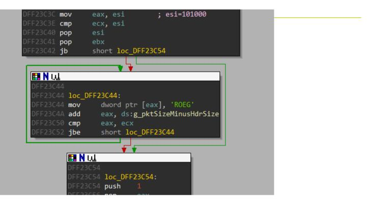
When reconstructing the BIOS image from the rbu packets, SMM writes an initialization string "GEOR" to the destination memory space where the BIOS image is being reconstructed....
