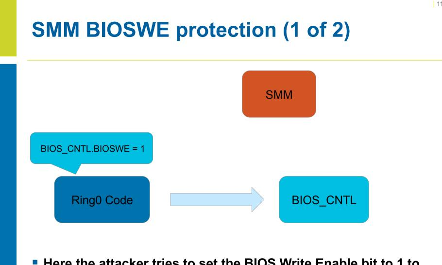
Here the attacker tries to set the BIOS Write Enable bit to 1 to allow him to overwrite the BIOS chip.
