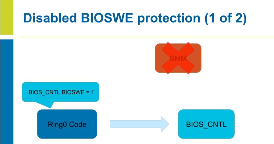
Again the attacker tries to set the BIOS Write Enable bit to 1 to allow him to overwrite the BIOS chip.
