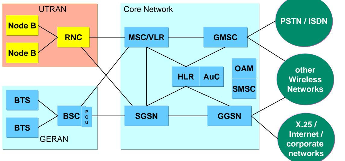
Source: 3GPP RAN: Radio Access Network **RNC: Radio Network Controller** AuC: Authentication Center MSC: Mobile Switching Center UTRAN: UMTS RAN BTS: Base Transceiver Station VLR: Visitor Location Register **OAM: Operation Administration & Maintenance GERAN: GSM Enhanced RAN BSC: Base Station Controller GMSC: Gateway MSC** SMSC: Short Message Service Center PCU: Paket Control Unit HLR: Home Location Register **GSN: GPRS Support Node** S/GGSN: Serving/Gateway GSN
